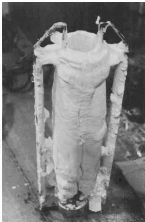
Fig. 5. Appearance of polymer deposit on scraping blades after stopping the recycle of heavy phase (runs 22–24).
